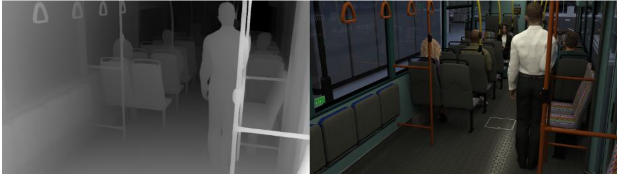
Figure 33: (left) depth image generated from a generative AI model (right) Image generated from photorealistic simulator.
