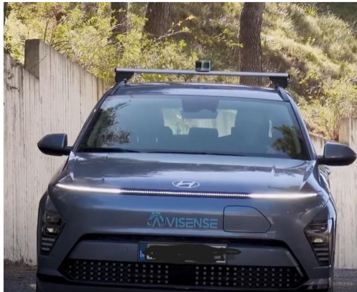
Figure 5: The Velodyne VLP-16 LiDAR sensor, as deployed on AVISENSE vehicles, provides 360-degree environmental perception with 16 vertical channels, enabling real-time 3D mapping and object detection.
