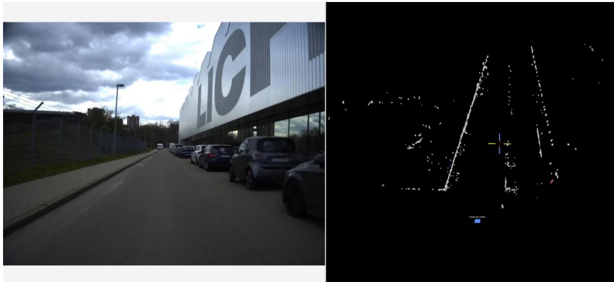
Figure 11: Point cloud data provided by the imaging radar visualized in Foxglove Studio
