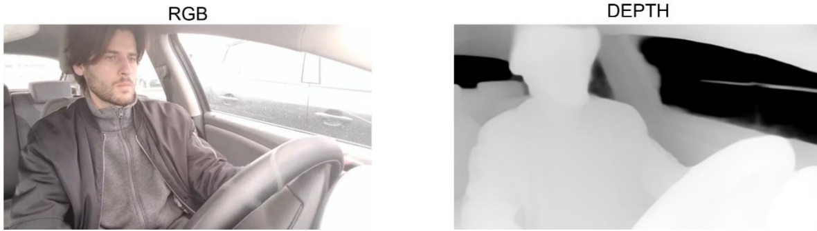
Figure 3: Example RGB and Depth output from the D435
